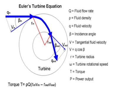
Power  $P = \omega T = \omega \rho Q(r_{in}q_{in} cos\beta_{in} - r_{out}q_{out} cos\beta_{out})$
